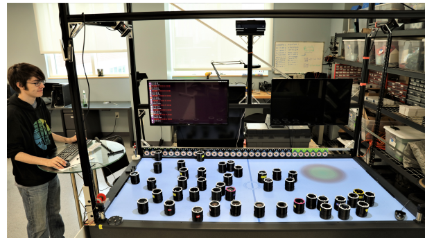
Fig. 1. Full system testing field of APIS with a human operator modifying the simulated environment using the overhead projector.
