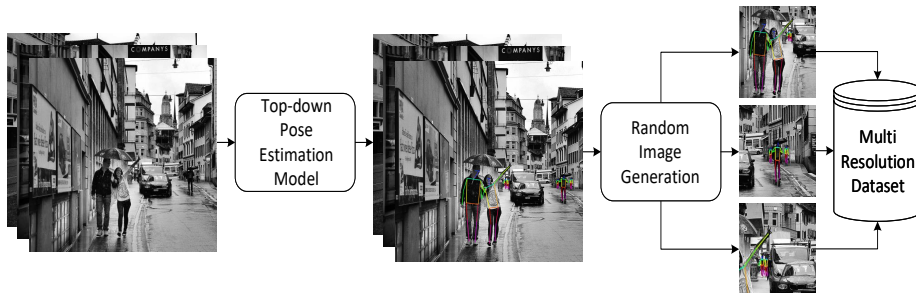
Fig. 2. Custom dataset generation. Beginning with ultra high resolution images, a pre-trained top-down pose estimation model is used to generate high accuracy keypoint annotations. Semi-random cropping is used to generate numerous high resolution images inline with user specified statistic, forming the new dataset.
